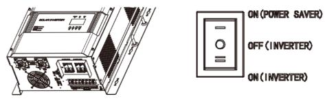
Once the unit has been properly installed and the batteries are connected well, simply press On/Off switch (located on the button of the case) to turn on the unit.
